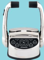
**Honda IST Intelligent Shift & Throttle - il sistema Honda "drive by wire"**
